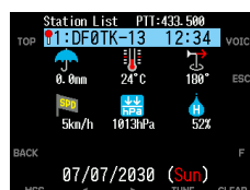
Weather station data including Rainfall, Temperature, Wind direction, Wind speed, Barometric pressure and Humidity
