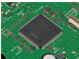
For IF DSP transmitter ADSP-21363 clock @ 332 MHz
